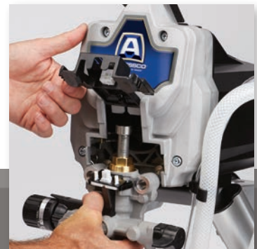
2. REMOVE PUMP SECTION
