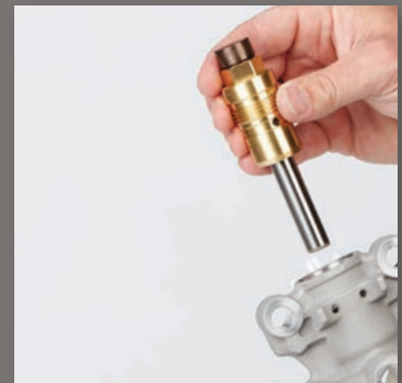
4. INSTALL NEW CARTRIDGE AND REPLACE PUMP
