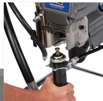
2. LIFT DOOR AND REMOVE PUMP
